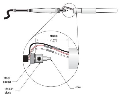
13. Remove any excess cable core, if necessary.
