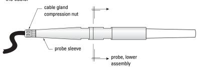
Unscrew the probe sleeve from the lower assembly using two 17 mm (0.67") wrenches across the flat surfaces, as shown below.
