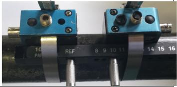
Install supplied 20' cables onto transducers. BNC connectors use a collar that must be pressed on and rotated to secure. Cables are marked UP and DN for upstream and downstream sensors:
