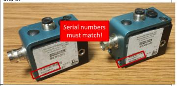
Unscrew thumb screws from spacer bar and use to space sensors based on Spacing Offset from [4]. Sensor BNC cable ports should face away from each other:
