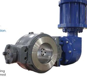
The 590's straight through unrestricted flow path provides higher capacity than globe style valves. A splined shaft provides accurate control in throttling operations and flexibility in actuation options. The 590 series, when combined with a Model DFRP piston actuator, is a rugged control valve assembly, to which a wide variety of positioners and accessories can be mounted.
