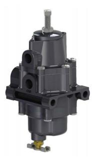
PRO-50 Series regulators are designed to be a compact, lightweight option for providing controlled and reduced pressures for instrumentation. Generally used to provide a constant supply pressure to pneumatic and electro-pneumatic controllers, these direct-operated regulators are rugged enough to be used in most air or gas applications.
