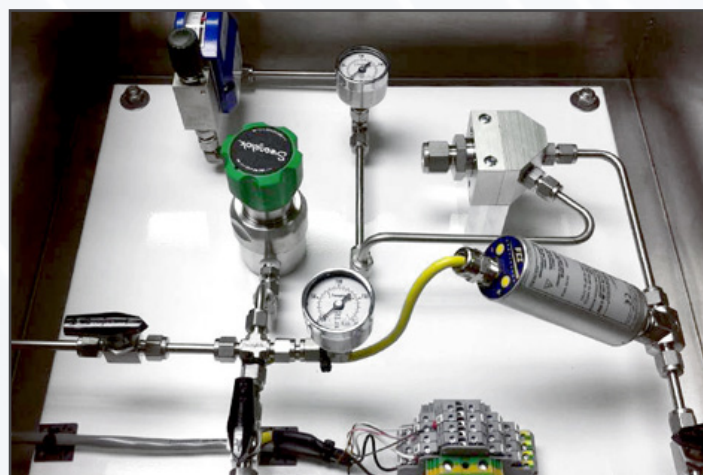
Figure 3: FCI Model FS10A in a typical sampling system
